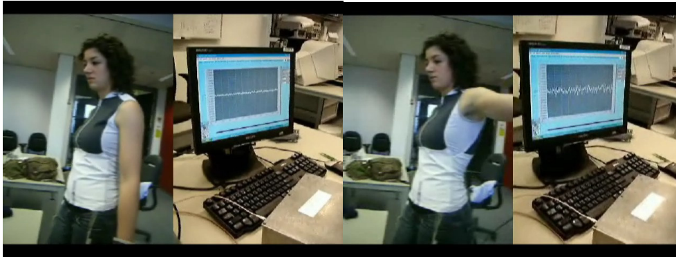
Figure 3. Researcher from the TNO is wearing the ConText prototype vest and taking turns of resting and 90 degrees abductions with her arms.
