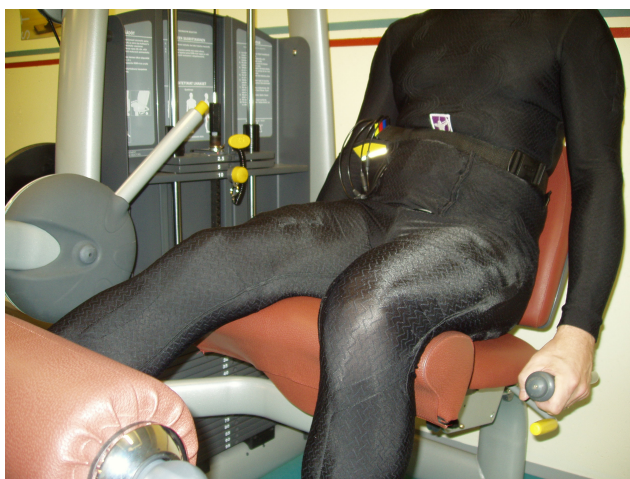
Figure 2. Testee person is wearing EMG trousers and shirt with textile electrodes.
